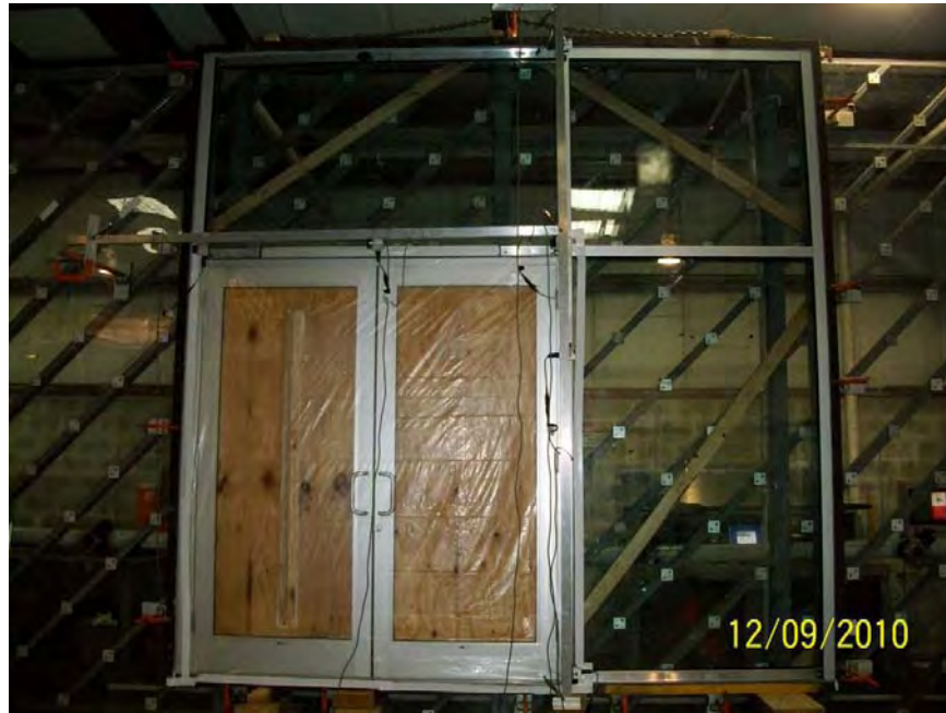
Photo No. 1 Elevation E5 Reinforced Captured Mullion with Series 381 Entrance Door
