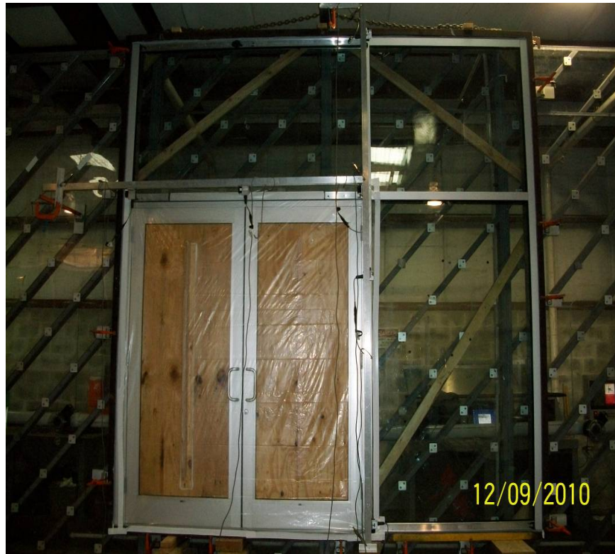
Photo No. 1 Elevation E5 Reinforced Captured Mullion with Series 381 Entrance Door
