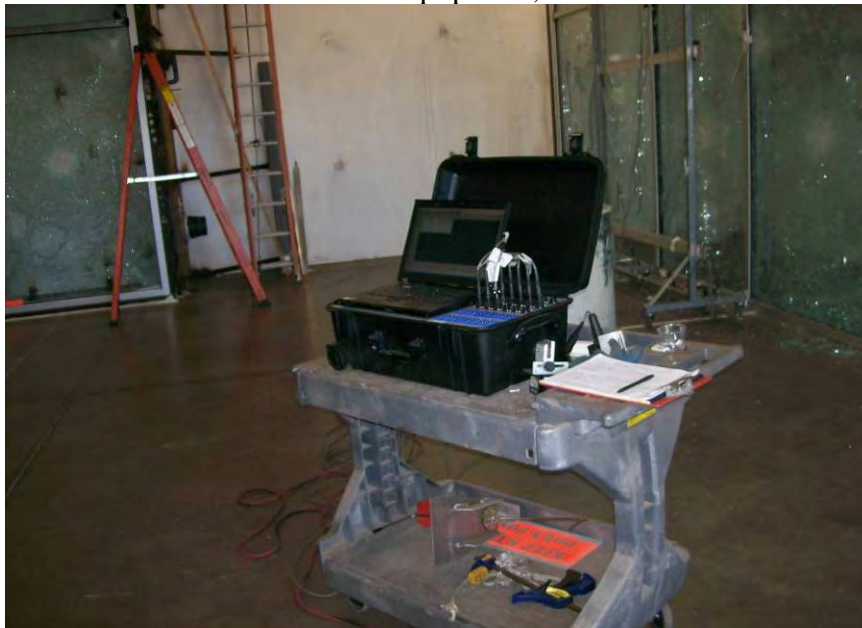
Photo No. 2 Deflection measuring equipment
