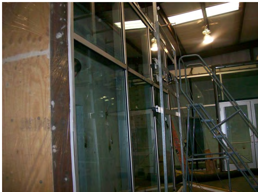
Photo No. 4 Specimen # 1 Set up for structural pressure test.
