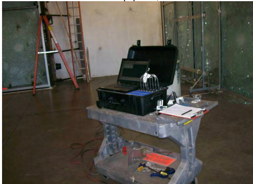
Photo No. 2 Deflection measuring equipment
