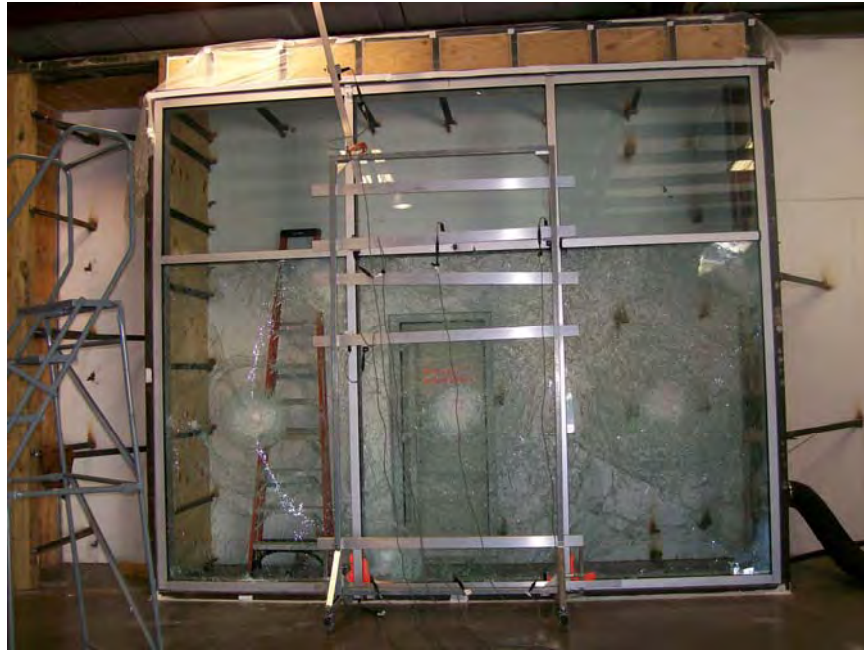
Photo No. 5 Specimen # 1, 2 and 3 Impact shots and set up for cyclic pressure test.
