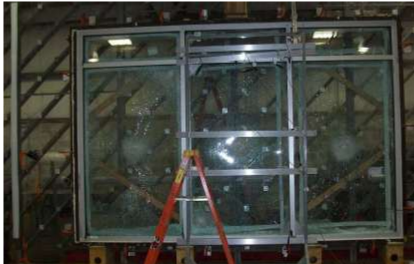
Photo No. 6 Specimens #1, #2 and #3 During TAS 203 Cyclic Loading
