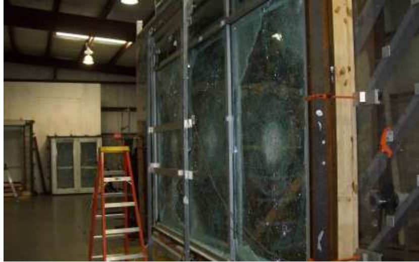
Photo No. 5 Specimens #1, #2, #3 Exterior View After TAS 201 and Before TAS 203 Cyclic Loading
