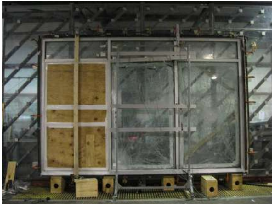
Photo No. 8 Specimens #1, #2, #3 Wood bracing was used on Specimen #1 in order to continue cyclic testing on Specimens #2 and #3
