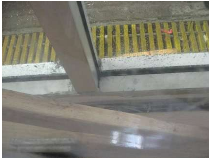
Photo No. 4 Specimens #2 and #3 Water accumulating in corners near glazing pocket during 15.04 psf water test
