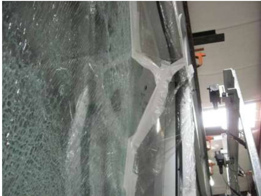
Photo No. 7 Specimen #1 Close-up of corner failure; glazing was pulled from glazing pocket
